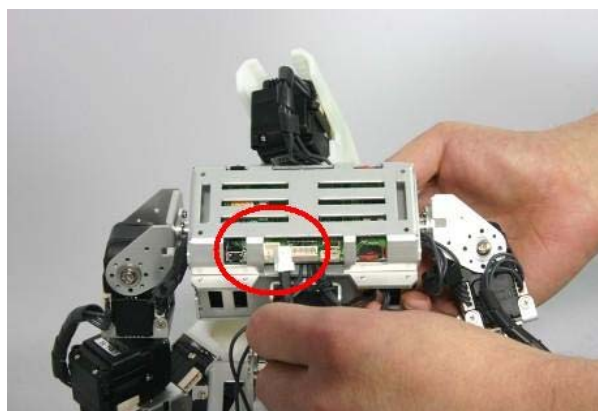
< Exterior power connection >
